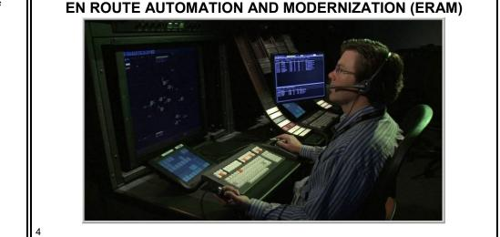
The ERAM system provides air traffic controllers with advanced tools to manage information and to facilitate interacting with that information.
